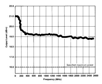
Typical output level. +19.9 dBm overrange setting.
